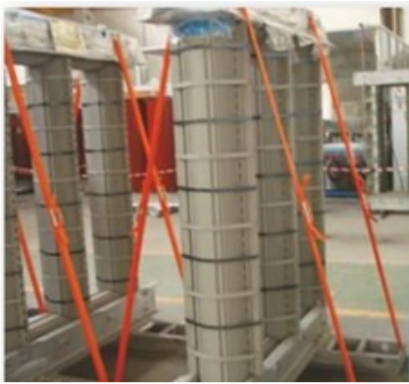
CRGO stacked assembled core
