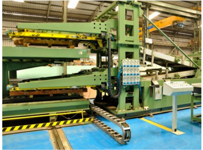
CNC Machine with cut to length and automatic stacking facility
